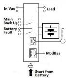
Input: Single-phase 115 - 277 Vac Output Load: power supply 48 Vdc; 10 A Output Battery: charging 48 Vdc; 10 A
